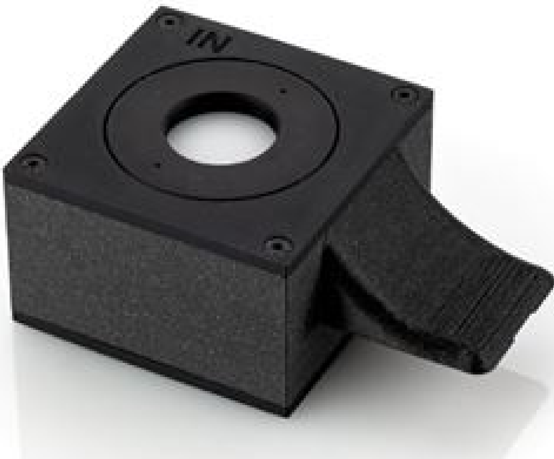
fNIRS Standard Phantom - IEC 80601-2-71
