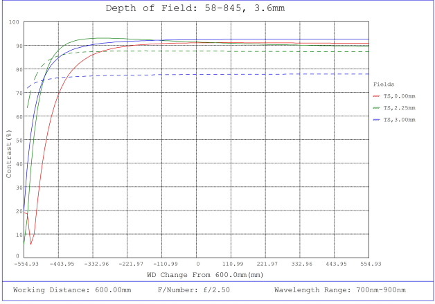
#58-845, f/2.5, NIR, 3.6mm HEO Series M12 Lens, Depth of Field Plot, 600mm Working Distance, f2.5
