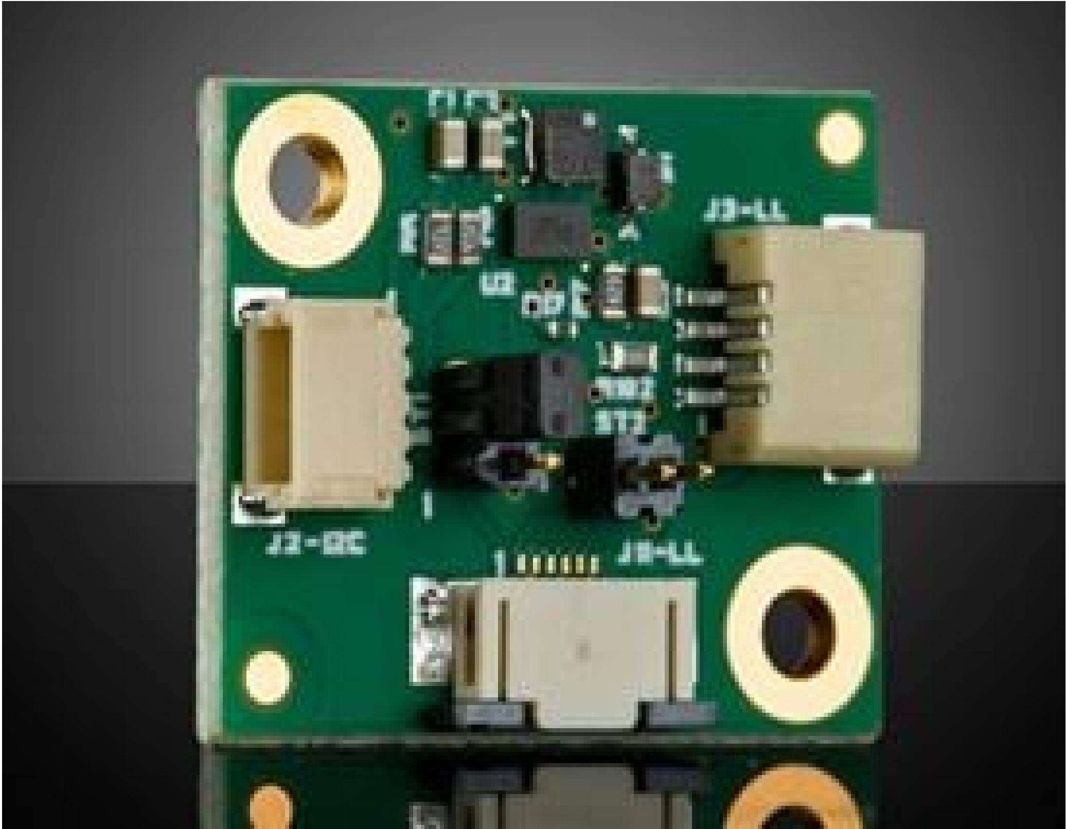
Corning® Varioptic® Variable Focus Liquid Lens Driver Board with Maxim MAX14574 Driver and I2C/DC Input
