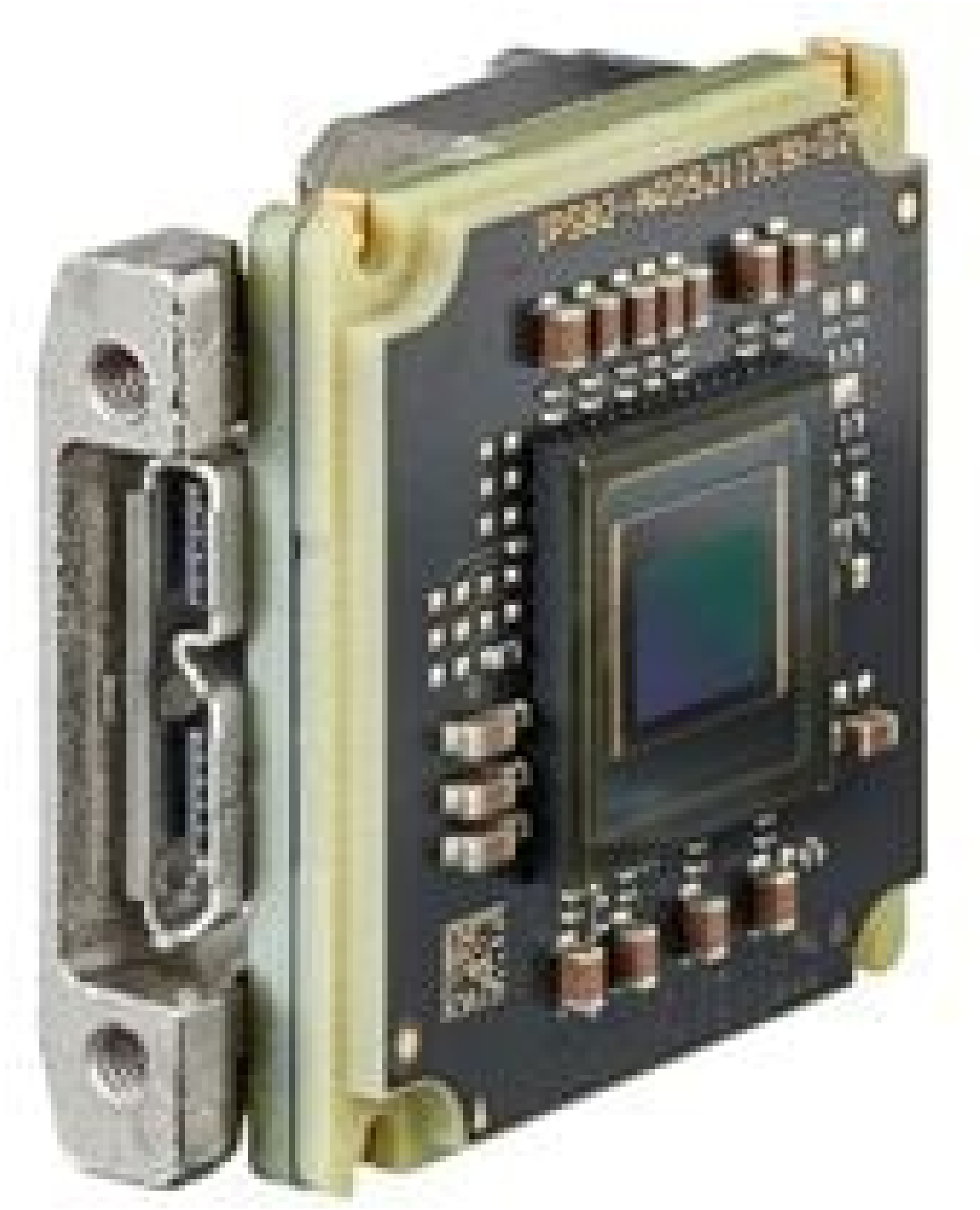
Allied Vsion Alvium Camera, Board Level, Right Angle IO Port (Front)
