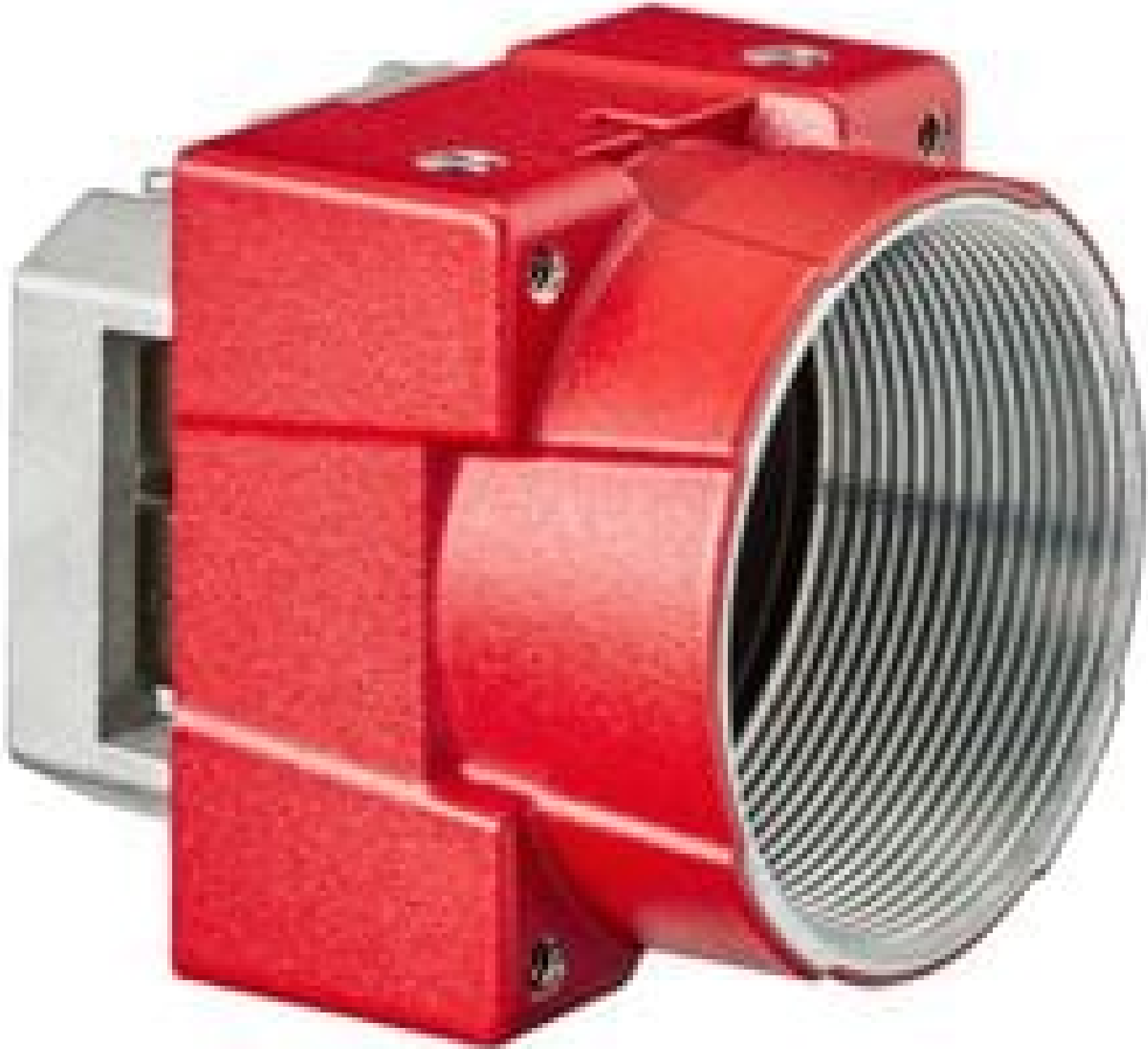
Allied Vision Alvium Camera, Partial Housing (Front)
