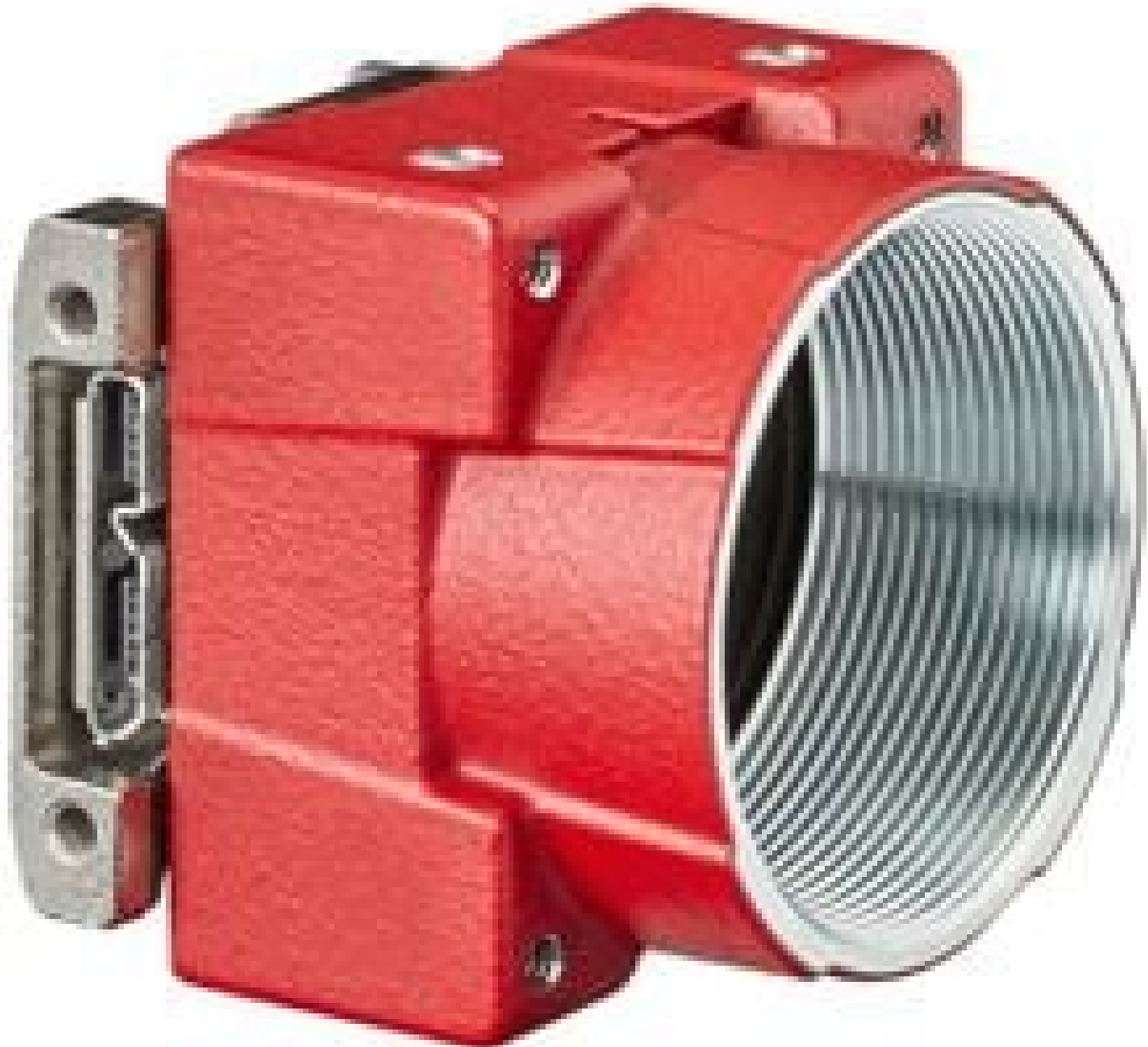
Allied Vision Alvium Camera, Partial Housing, Right Angle IO Port (Front)
