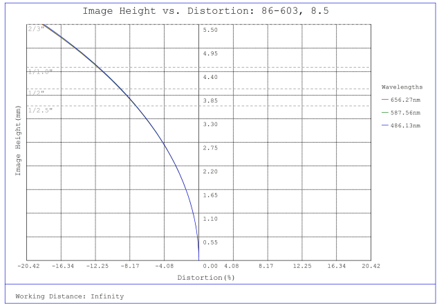
#86-603, 8.5mm, f/5.6 Ci Series Fixed Focal Length Lens, Distortion Plot
