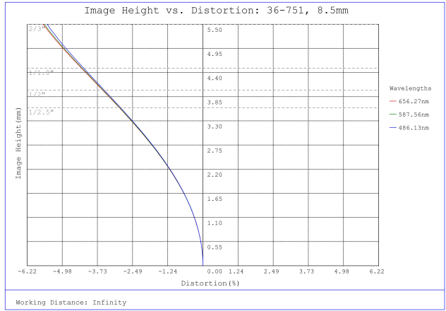
#36-751, 8.5mm f/5.6, 75mm-∞ Primary WD, HRi Series Fixed Focal Length Lens, Distortion Plot
