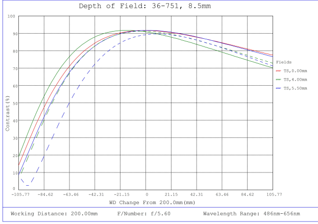
#36-751, 8.5mm f/5.6, 75mm-∞ Primary WD, HRi Series Fixed Focal Length Lens, Depth of Field Plot, 200mm Working Distance, f5.6
