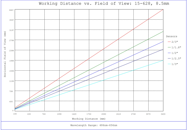
#15-628, 8.5mm, f/4 Cw Series Fixed Focal Length Lens, Working Distance versus Field of View Plot
