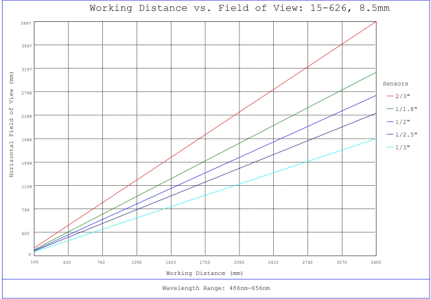
#15-626, 8.5mm, f/1.8 Cw Series Fixed Focal Length Lens, Working Distance versus Field of View Plot
