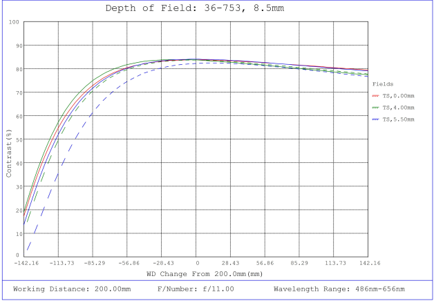
#36-753, 8.5mm f/11, 75mm-∞ Primary WD, HRi Series Fixed Focal Length Lens, Depth of Field Plot, 200mm Working Distance, f11
