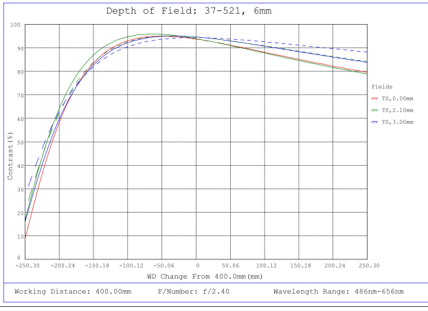
#37-521, 6mm FL, Liquid Lens M12 Lens, Depth of Field Plot, 400mm Working Distance, f2.4
