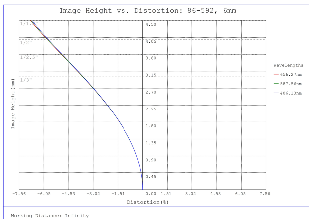
#86-592, 6mm, f/1.8 Ci Series Fixed Focal Length Lens, Distortion Plot
