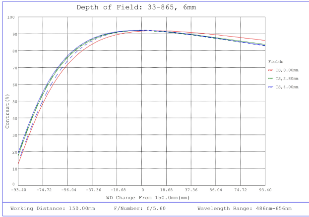
#33-865, 6mm, f/5.6 UCi Series Fixed Focal Length Lens, Depth of Field Plot, 150mm Working Distance, f5.6
