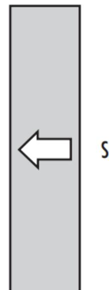
All mounted TECHSPEC® Optical Filters have an arrow on the side of the mount that points to the filter-coated surface for quick reference. Filter oriented such that arrow points to filter coated surface S1. Anti-reflective (AR) coating is applied to S2.
