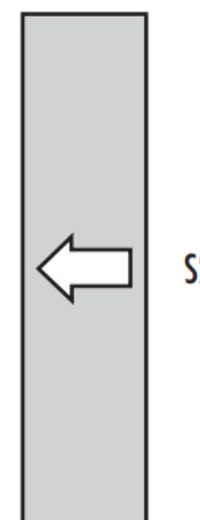
All mounted TECHSPEC® Optical Filters have an arrow on the side of the mount that points to the filter-coated surface for quick reference. Filter oriented such that arrow points to filter coated surface S1. Anti-reflective (AR) coating is applied to S2.
