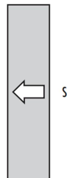
All mounted TECHSPEC® Optical Filters have an arrow on the side of the mount that points to the filter-coated surface for quick reference. Filter oriented such that arrow points to filter coated surface S1.
