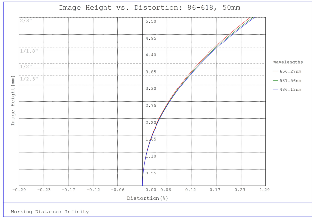
#86-618, 50mm, f/8.0 Ci Series Fixed Focal Length Lens, Distortion Plot
