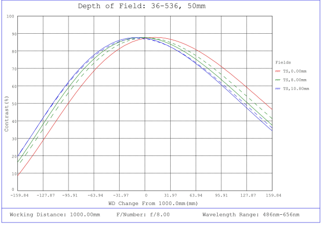
#36-536, 50mm f/8.0, HPr Series Fixed Focal Length Lens, Depth of Field Plot, 1000mm Working Distance, f8
