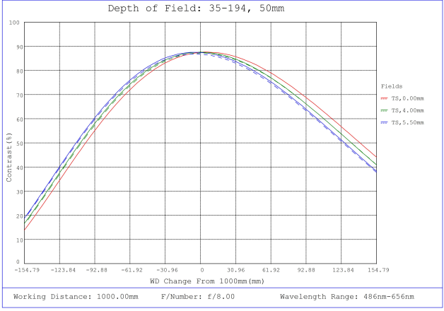
#35-194, 50mm, f/8.0 Cr Series Fixed Focal Length Lens, Depth of Field Plot, 1000mm Working Distance, f8
