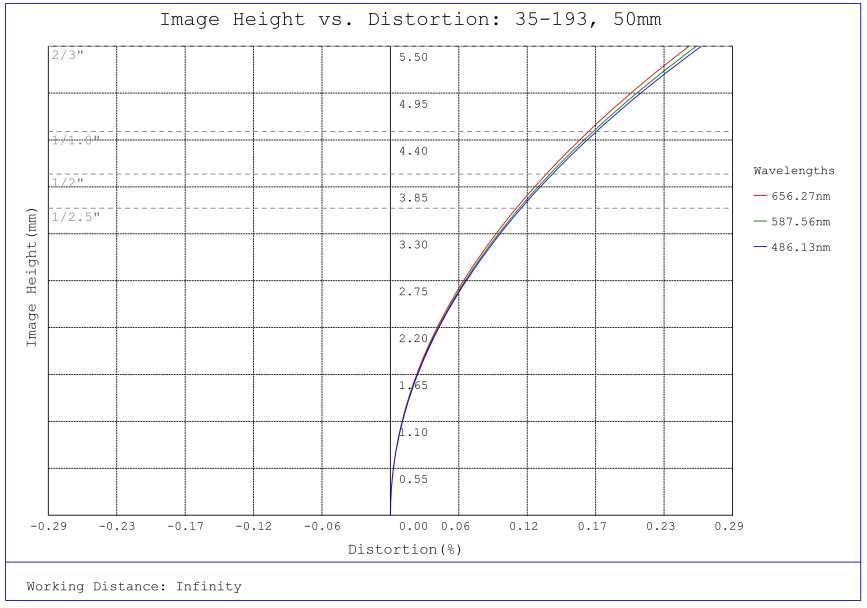
#35-193, 50mm, f/5.6 Cr Series Fixed Focal Length Lens, Distortion Plot
