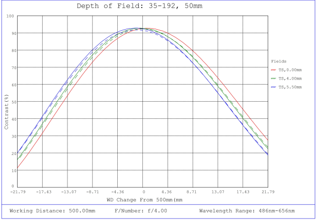
#35-192, 50mm, f/4.0 Cr Series Fixed Focal Length Lens, Depth of Field Plot, 500mm Working Distance, f4
