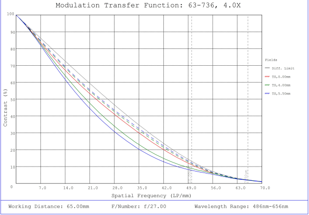
#63-736, 4X, 65mm WD CompactTL™ Telecentric Lens, Modulated Transfer Function (MTF) Plot, 65mm Working Distance, f27
