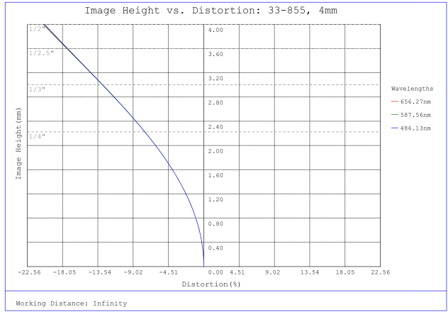
#33-855, 4mm, f/1.8 UCi Series Fixed Focal Length Lens, Distortion Plot
