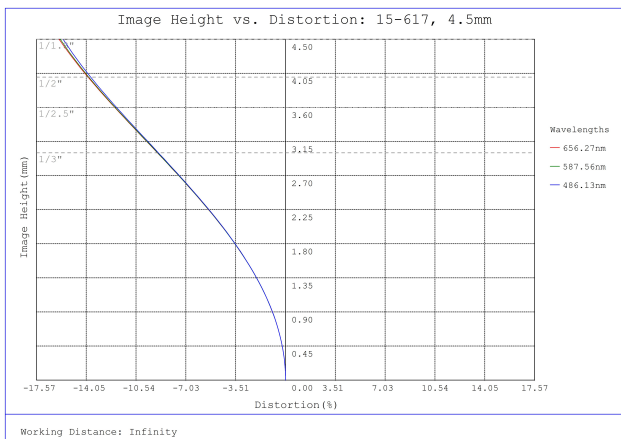
#15-617, 4.5mm f/8.0 Sealed Cw Series Fixed Focal Length Lens, Distortion Plot
