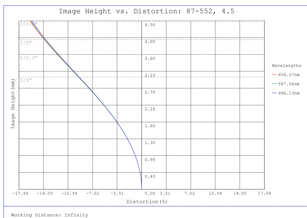
#87-552, 4.5mm, f/2.8 Ci Series Fixed Focal Length Lens, Distortion Plot
