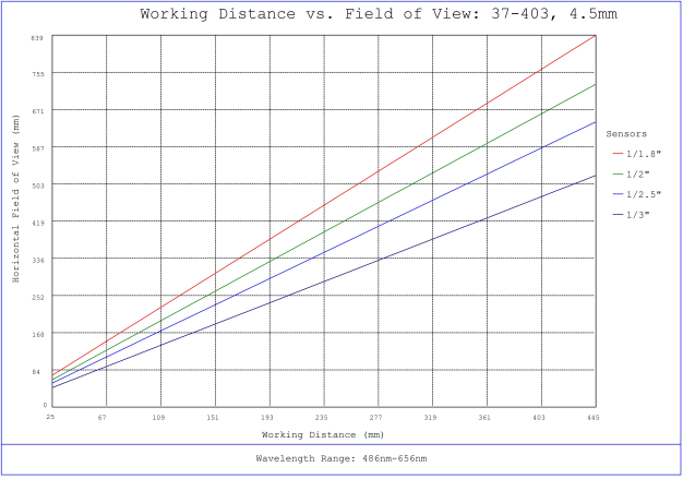
#37-403, 4.5mm, f/11 Cr Series Fixed Focal Length Lens, Working Distance versus Field of View Plot
