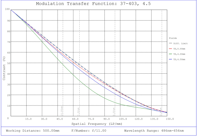
#37-403, 4.5mm, f/11 Cr Series Fixed Focal Length Lens, Modulated Transfer Function (MTF) Plot, 500mm Working Distance, f11
