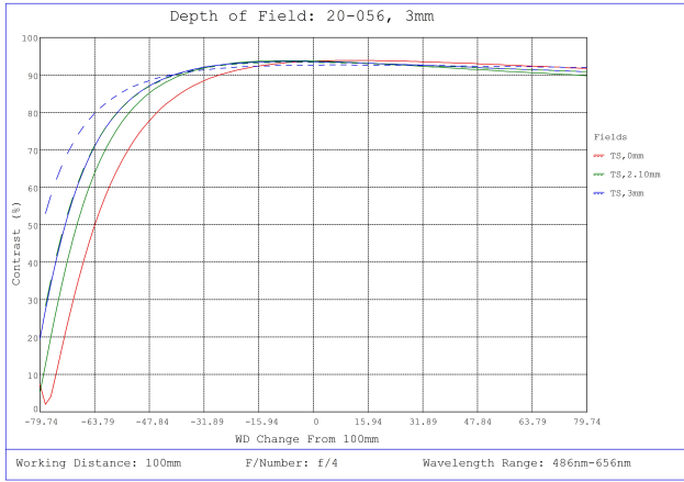
#20-056, 3mm FL f/4.0, IR-Cut Blue Series M12 Lens, Depth of Field Plot, 100mm Working Distance, f4
