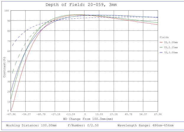
#20-059, 3mm FL f/2.5 IR-Cut Rugged Blue Series M12 Lens, Depth of Field Plot, 100mm Working Distance, f2.5
