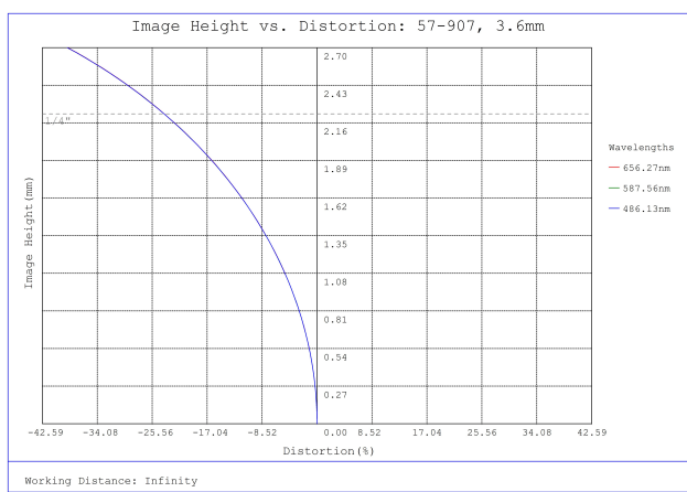
#57-907, 3.6mm FL, Red Series M12 Lens, Distortion Plot
