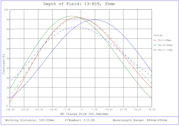
#13-809, 35mm TFL-II Mount LH Series Fixed Focal Length Lens, Depth of Field Plot, 500mm Working Distance, f2.8
