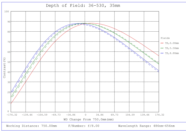
#36-530, 35mm f/8.0, HPr Series Fixed Focal Length Lens, Depth of Field Plot, 750mm Working Distance, f8
