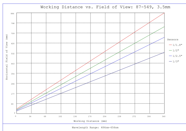
#87-549, 3.5mm, f/8 Ci Series Fixed Focal Length Lens, Working Distance versus Field of View Plot
