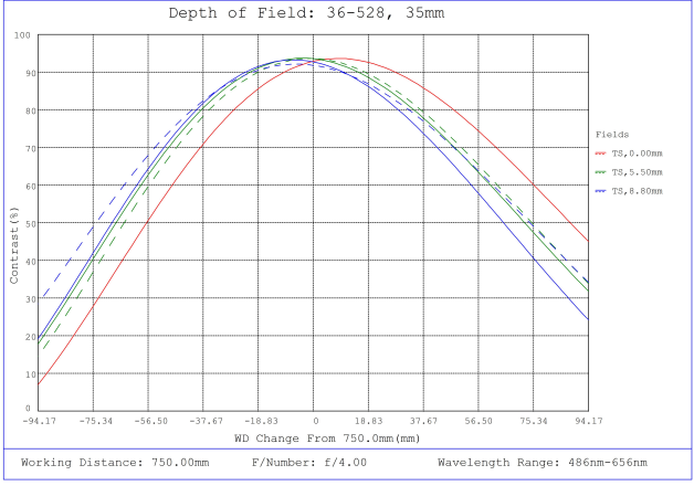
#36-528, 35mm f/4.0, HPr Series Fixed Focal Length Lens, Depth of Field Plot, 750mm Working Distance, f4
