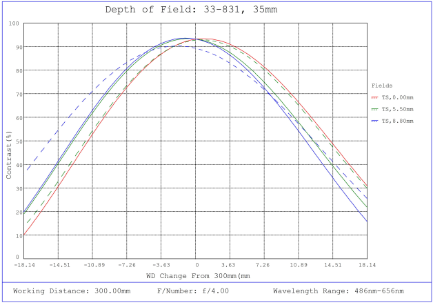
#33-831, 35mm f/4.0, HPi Series Fixed Focal Length Lens, Depth of Field Plot, 300mm Working Distance, f4
