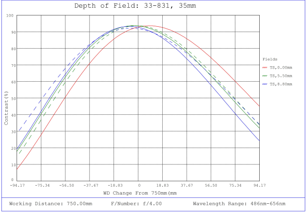
#33-831, 35mm f/4.0, HPi Series Fixed Focal Length Lens, Depth of Field Plot, 750mm Working Distance, f4
