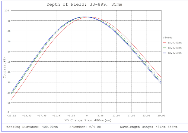
#33-899, 35mm f/4, UCI Series Fixed Focal Length Lens, Depth of Field Plot, 400mm Working Distance, f4
