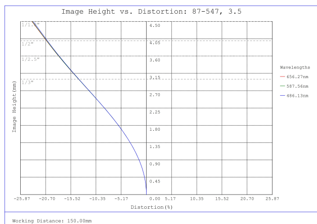
#87-547, 3.5mm, f/4 Ci Series Fixed Focal Length Lens, Distortion Plot
