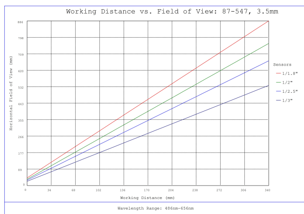
#87-547, 3.5mm, f/4 Ci Series Fixed Focal Length Lens, Working Distance versus Field of View Plot
