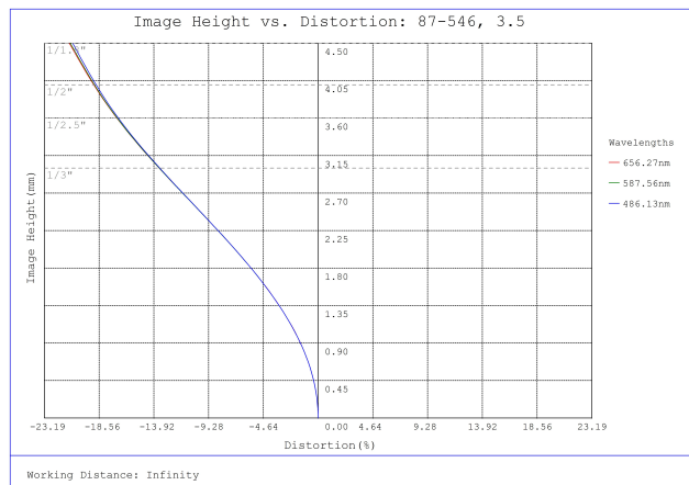
#87-546, 3.5mm, f/2.8 Ci Series Fixed Focal Length Lens, Distortion Plot
