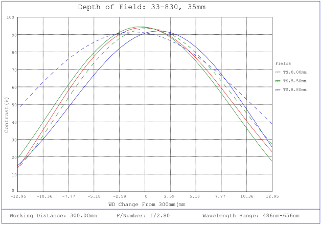
#33-830, 35mm f/2.8, HPi Series Fixed Focal Length Lens, Depth of Field Plot, 300mm Working Distance, f2.8
