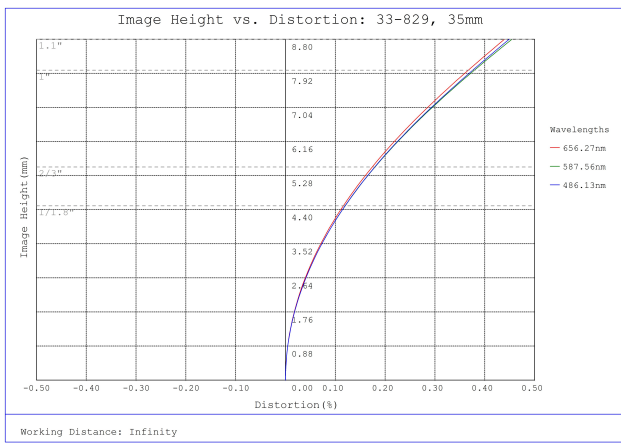
#33-829, 35mm f/2.0, HPI Series Fixed Focal Length Lens, Distortion Plot
