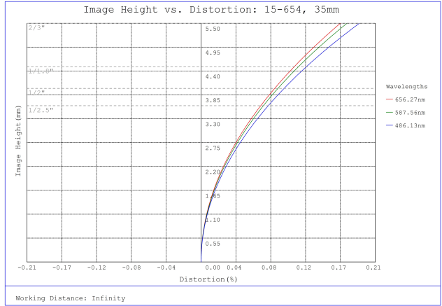
#15-654, 35mm, f/1.65 Cw Series Fixed Focal Length Lens, Distortion Plot
