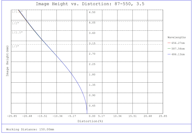
#87-550, 3.5mm, f/11 Ci Series Fixed Focal Length Lens, Distortion Plot
