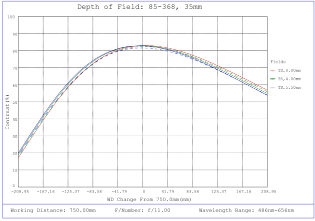
#85-368, 35mm, f/11 Ci Series Fixed Focal Length Lens, Depth of Field Plot, 750mm Working Distance, f11
