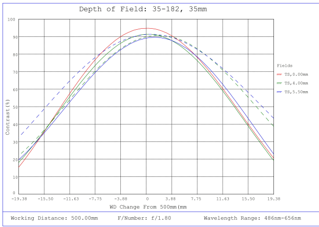
#35-182, 35mm, f/1.8 Cr Series Fixed Focal Length Lens, Depth of Field Plot, 500mm Working Distance, f1.8
