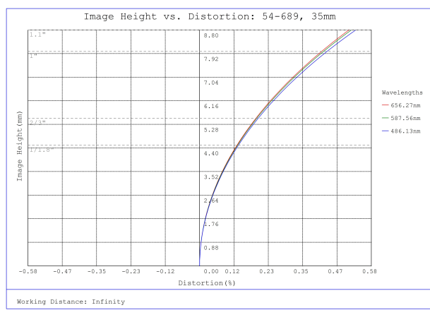
#54-689, 35mm DG Series Fixed Focal Length Lens, Distortion Plot
