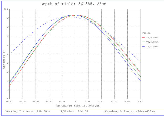
#36-385, 25mm FL f/4, Rugged Blue Series M12 Lens, Depth of Field Plot, 150mm Working Distance, f4
