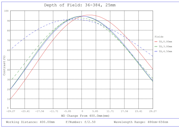
#36-384, 25mm FL f/2.5, Rugged Blue Series M12 Lens, Depth of Field Plot, 400mm Working Distance, f2.5
