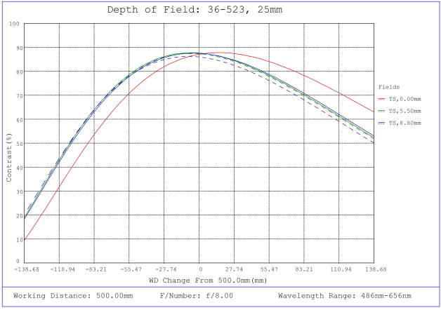
#36-523, 25mm f/8.0, HPr Series Fixed Focal Length Lens, Depth of Field Plot, 500mm Working Distance, f8
