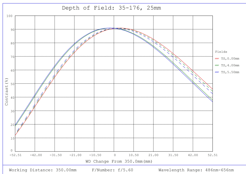
#35-176, 25mm, f/5.6 Cr Series Fixed Focal Length Lens, Depth of Field Plot, 350mm Working Distance, f5.6
