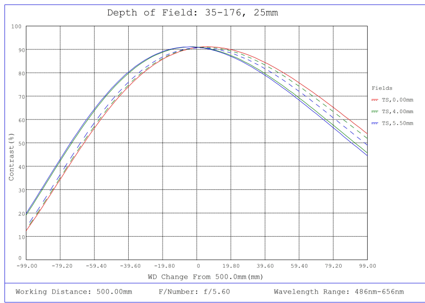
#35-176, 25mm, f/5.6 Cr Series Fixed Focal Length Lens, Depth of Field Plot, 500mm Working Distance, f5.6
