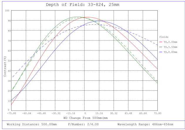
#33-824, 25mm f/4.0, HPi Series Fixed Focal Length Lens, Depth of Field Plot, 500mm Working Distance, f4
